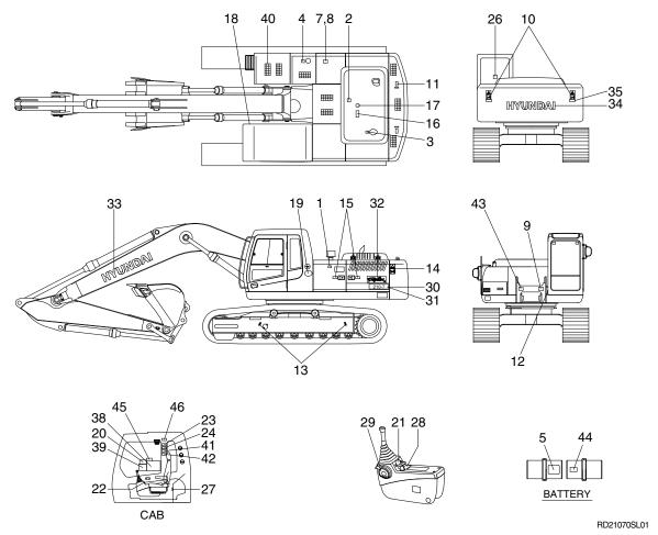
1 Air cleaner filter 2 Turbo charger cover 3 Radiator cap 4 **Fueling** 5 Battery accident 7 Hydraulic oil level 8 Hydraulic oil lubrication 9 Reduction gear grease 10 Keep clear 11 Lifting eye 12 Name plate 13 Slinging ideogram 14 Sidekeep clear
